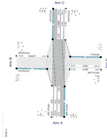
Showing modelled flow through junction (PCU/hr).
